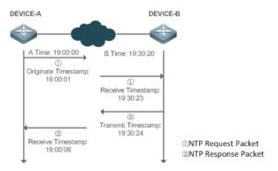
DEVICE-B (B for short) is used as an NTP reference clock source, DEVICE-A (A for short) is used as an NTP client that synchronizes time with DEVICE-B. At a time point, the local clock of A is 19:00:00 and the local clock of B is 19:30:20.
