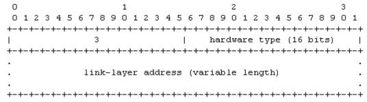
The values of *DUID-LL*, *Hardware type*, and *Link-layer address* are 0x0003, 0x0001 (indicating the Ethernet), and MAC address of a device respectively.
