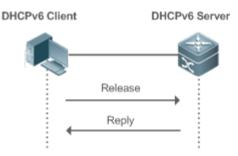
After receiving the Release message, the DHCPv6 server removes the corresponding bindings based on the addresses
