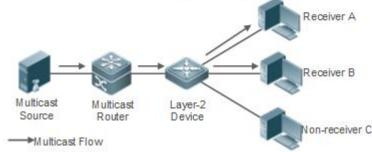
As shown in the following figure, when IGMP Snooping does not run on the AC and AP in wireless multicast environment, multicast packets are broadcasted within the VLAN of the AC and are broadcasted by the AP to all wireless ports. When IGMP Snooping runs on both the AC and AP, multicast packets of a known multicast profile are not broadcasted but forwarded to specific receivers.
