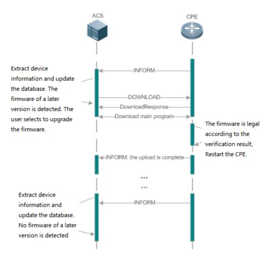
Users specify a CPE for the ACS to deliver the Download method for upgrading the firmware. The CPE receives the request and starts to download the latest firmware from the destination file server, upgrade the firmware, and then reboot. After restart, the CPE will indicate the successful or unsuccessful completion of the method application.
