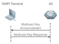
After the unicast key negotiation succeeds, that is, a unicast key security association is established, the AE sends a multicast key announcement to the ASUE to notify the ASUE of the key used by the AE for sending multicast data.
