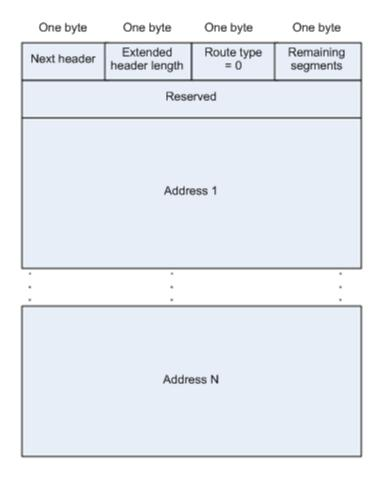
The following example describes the application of the Type 0 routing header, as shown in Figure 3-15.
