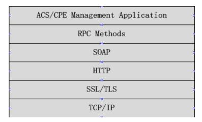
As shown in Figure 9-2, CWMP defines six layers with respective functions as follows:
