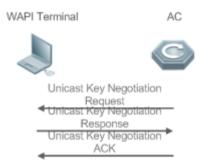
After the certificate authentication succeeds, the AE sends a key negotiation request to the ASUE, containing the key negotiation request data.
