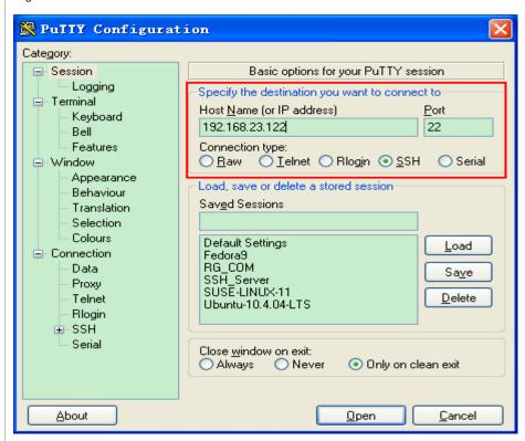
**Host Name (or IP address)** indicates the IP address of the host to be logged in. In this example, the IP address is **192.168.23.122**. **Port** indicates the port ID 22, that is, the default ID of the port listened by SSH. **Connection type** is **SSH**.
