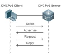
A DHCPv6 client sends a Solicit message whose destination address is FF02::1:2 and destination port number is 547 within the local link to request address, prefix and configuration parameter allocation. All DHCPv6 servers or DHCPv6 relay agents within the link will receive the Solicit message.
