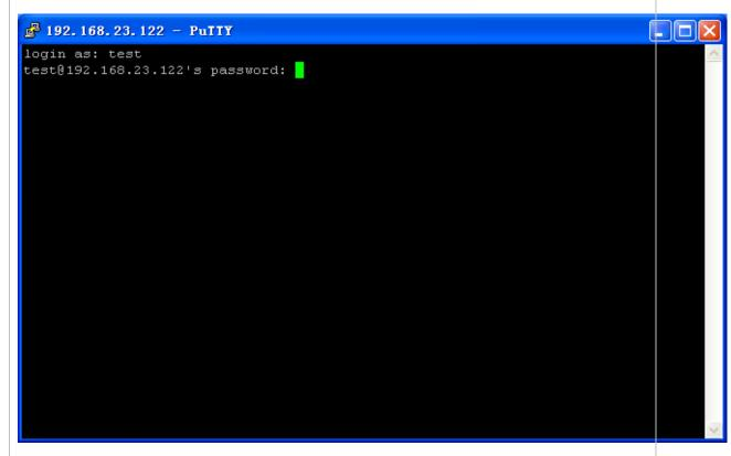
Type in the correct user name and password, and you can log in to the SSH terminal interface, as shown in Figure 15-10.
