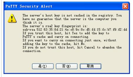
The **Putty Security Alert** box indicates that you are logging in to the client of the server 192.168.23.122, and asks you whether to receive the key sent from the server.
