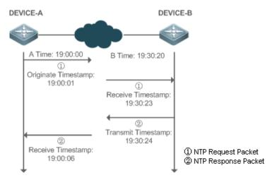
DEVICE-B (B for short) is used as an NTP reference clock source, DEVICE-A (A for short) is used as an SNTP client that synchronizes time with DEVICE-B. At a time point, the local clock of A is 19:00:00 and the local clock of B is 19:30:20.
