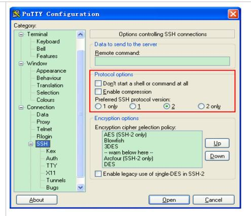
As shown in Figure 15-7, select **2** as the preferred SSH protocol version in the **Protocol options** pane because SSHv2 is used for login.
