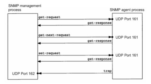
The three operations performed by the NMS on the agent and the response operations of the agent are based on UDP port 161. The trap operation performed by the agent is based on UDP port 162.
