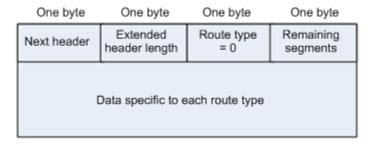
The Segments Left field is used to indicate how many intermediate nodes are specified in the routing header for the packet to pass through from the current node to the final destination address.
