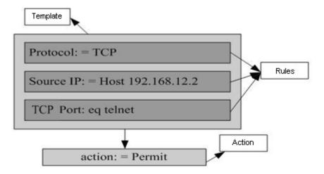
A filtering field template can be a combination of L3 and L4 fields, or a combination of multiple L2 fields. The filtering field template of a standard or an extended ACL, however, cannot be a combination of L2 and L3 fields, a combination
