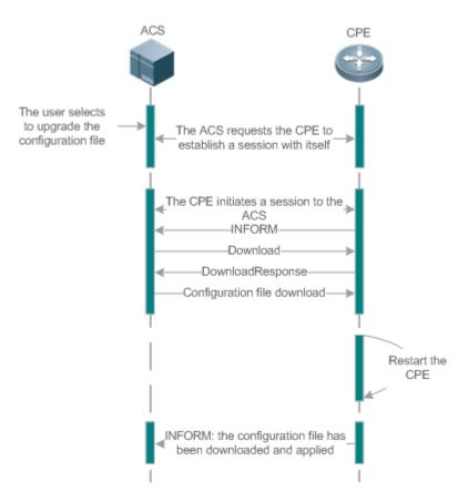
Users specify a CPE for the ACS to deliver the Download methods for upgrading its configuration files. The CPE downloads the configuration files from the specified file server, upgrade configuration files, and then reboot. After that, the CPE will indicate successful or unsuccessful completion of the method application.
