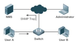
After MAC address change notification is enabled on a device, the device generates a notification message when the device learns a new MAC address or finishes aging a learned MAC address, and sends the message in an SNMP Trap message to a specified NMS.
