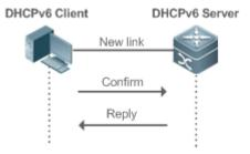
• After receiving the Confirm message, the DHCPv6 server performs confirmation based on the address information in the Confirm message, and sends a Reply message carrying the state option to the DHCPv6 client. If the confirmation fails, the DHCPv6 client may initiate a new address allocation request.
