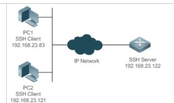
SSH users can use the local line password for user authentication, as shown in Figure 15-12.To ensure security of data exchange, PC 1 and PC 2 function as the SSH clients, and use the SSH protocol to log in to the network device where the SSH server is enabled. The requirements are as follows:
