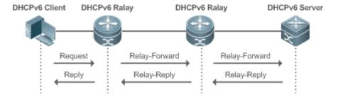
The DHCPv6 relay agent performs message encapsulation and decapsulation between the DHCPv6 client and DHCPv6 server to enable communication between the DHCPv6 client and DHCPv6 server on different links.
