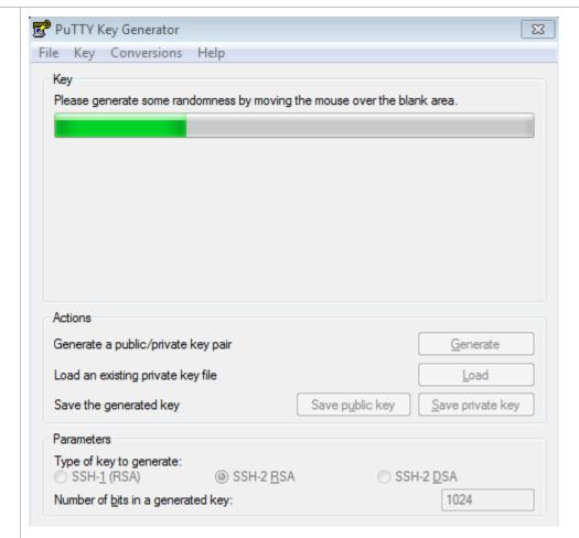
To ensure security of the RSA public key authentication, the length of the generated RSA key pair must be equal to or larger than 768 bits. In this example, the length is set to 1024 bits.
