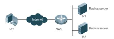
Figure 2-3 shows a typical AAA network topology, where two RADIUS servers (R1 and R2) and one NAS are deployed. The NAS can be the client for the RADIUS servers.
