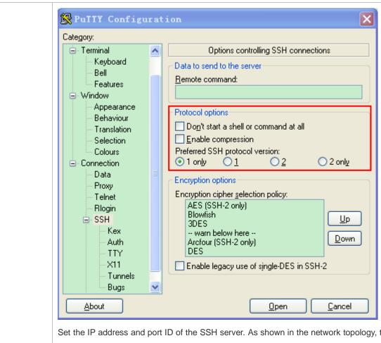
Set the IP address and port ID of the SSH server. As shown in the network topology, the IP address of the server is 192.168.23.122, and the port ID is 22 (For details about the configuration method, see "Configuring SSH Device Management."). Click **Open** to start the SSH server. As the current authentication mode does not require a user name, you can type in any user name, but cannot leave the user name unspecified. (In this example, the user name is "anyname".)
