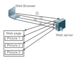
HTTP/1.1 overcomes the defect. It supports persistent connection, that is, one connection can be used to transmit multiple requests and response messages. In this way, a client can send a second request without waiting for completion of the previous request. This reduces network delay and improves performance. See the following figure:
