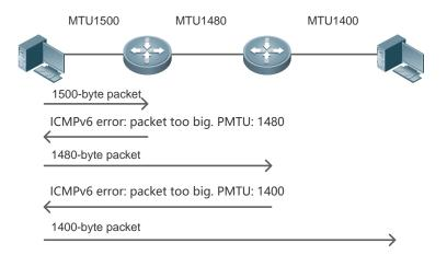
As shown in Figure 3-10, if the length of a packet to be sent by the host is greater than the PMTU, the router discards this packet and sends an ICMPv6 Packet Too Big message containing its PMTU to the host. The host then fragments the packet based on the new PMTU. In this manner, the router does not need to perform fragmentation, saving router resources and improving the IPv6 network efficiency.
