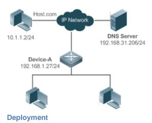
Deploy DNS Server as the DNS server of Device-A.
